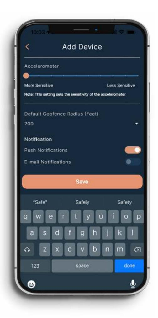
You can set the sensitivity of the motion detection using the slider bar. You can also set the geofence which sets up an area that if the device leaves, will trigger an alert. You can also select how you want to be notified. We recommend that you start with the default settings and edit them later in the Device tab area if needed. Click the Save button.
